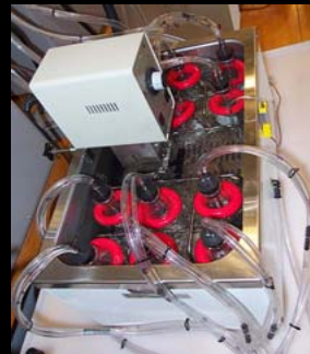
Water condenser and ammonia trap (9° C.)
