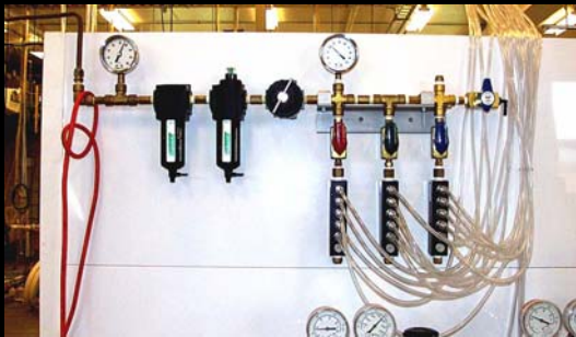
Flow restrictor system (air 100 \pm 3 ml/min)
